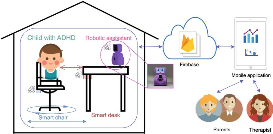
**Fig. 1.** Schematic of the SmartHome environment designed for pervasive occupational therapy for children with ADHD. This depiction shows the placement of various sensor devices and the robotic assistant within the house. These tools capture detailed information about the workspace, which is then relayed to Firebase for processing. The processed data can subsequently be accessed and visualized by therapists and parents via the mobile application developed in the course of this research.
